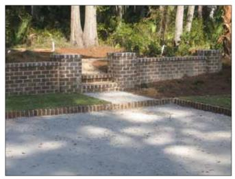
Crushed gravel parking area with brick edging
