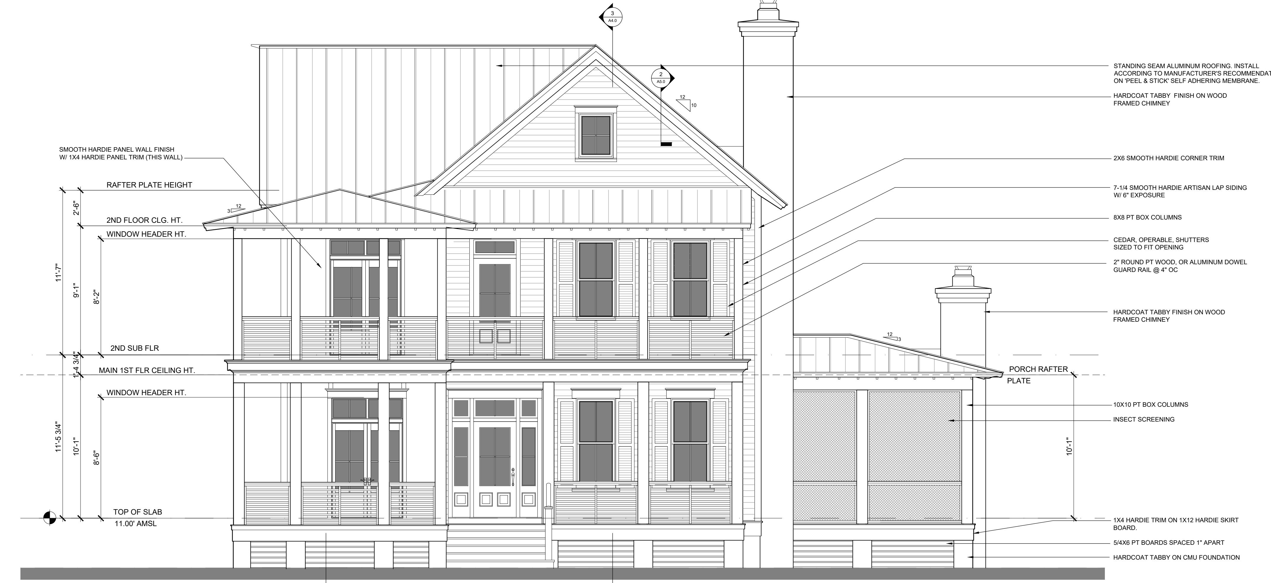
FINISH GRADE LINES SHOWN ARE APPROXIMATE. VERIFY THAT FINISHED GRADE SLOPES AWAY FROM BUILDING AT LEAST 4'-0", BUT NOT ON TO ADJACENT PROPERTIES. BUILDER SHALL ESTABLISH FINISHED FLOOR ELEVATION IN ACCORDANCE WITH LOCAL CODES. BUILDER SHALL ALSO MAINTAIN ADEQUATE CLEARANCE BETWEEN FINISHED GRADE AND ANY WOOD CONSTRUCTION. NUMBER OF STEPS TO GRADE DEPEND ON SPECIFIC SITE ELEVATIONS.
